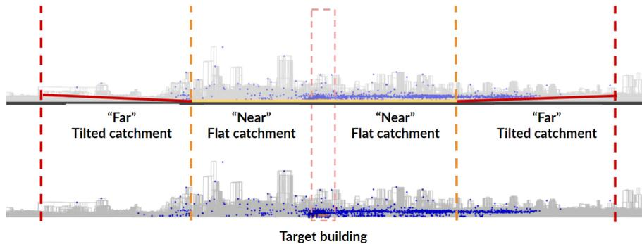
Figure 6. Sectional view diagram of context catchment area.
