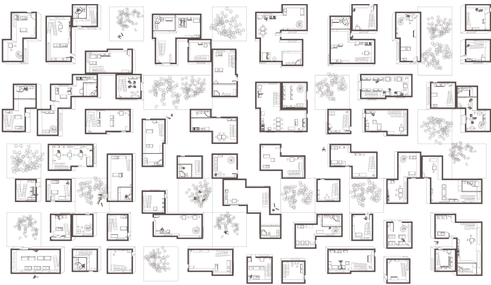
Figure 6. Floor plan generated using the spatial rules.
